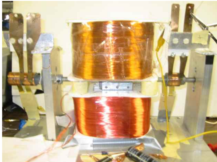
This is our Air Core Motor Design which can also be used for HFG9 generator.
